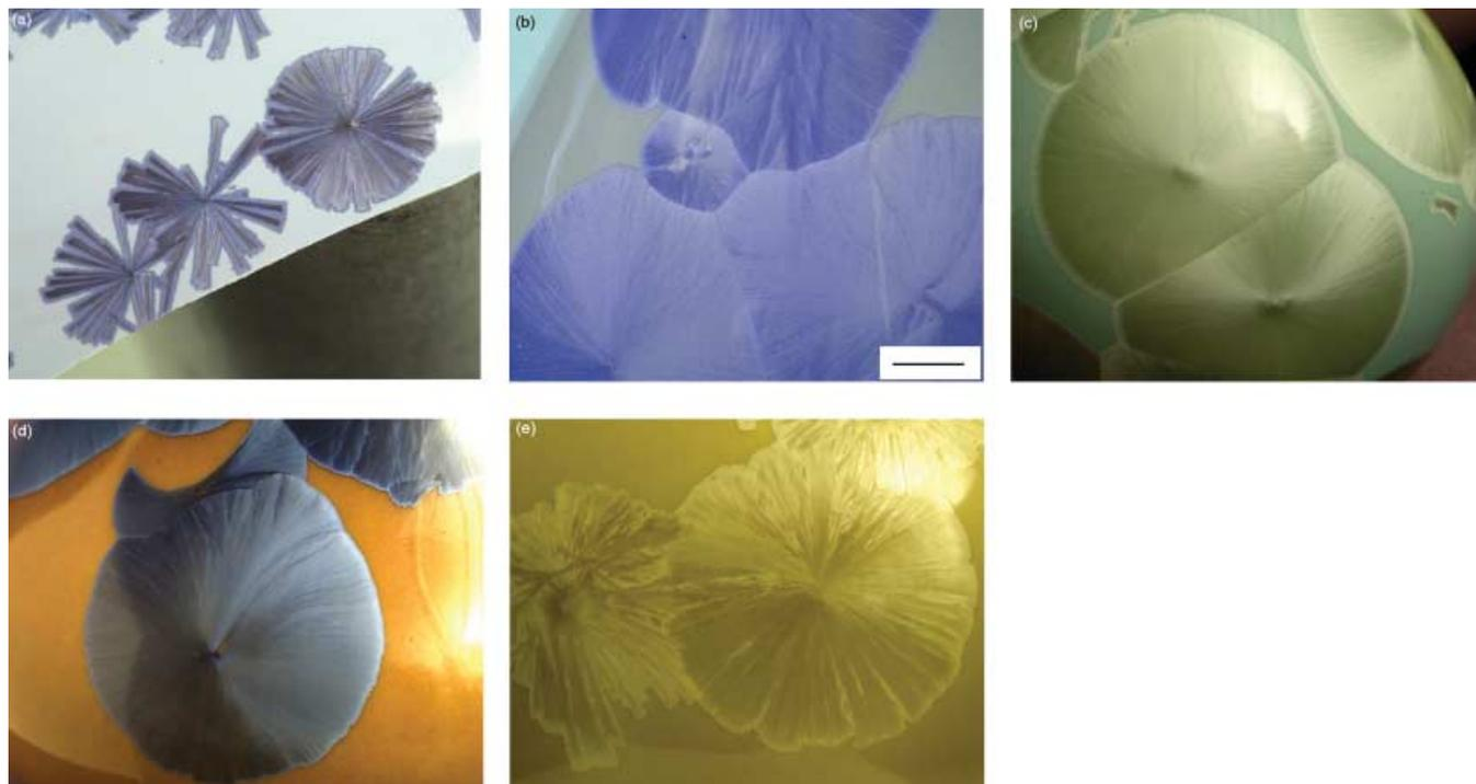
Fig. 2. (a)–(e) Reflected light micrographs of spherulites in P1–P5, respectively. The scale bar for all the micrographs shown in (b) is 5 mm. The spherulites in (a) are at the edge of an as-received broken piece from P1. This edge runs from the middle of the right-hand side of (a) to near the bottom left-hand corner of (a).
