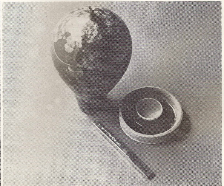
8. The completed form may be smoothed further at the foot with emery paper.
