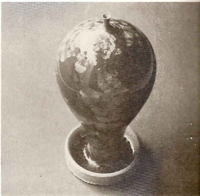
6. After firing, glaze has pooled in the bowl below the base of the ware.
