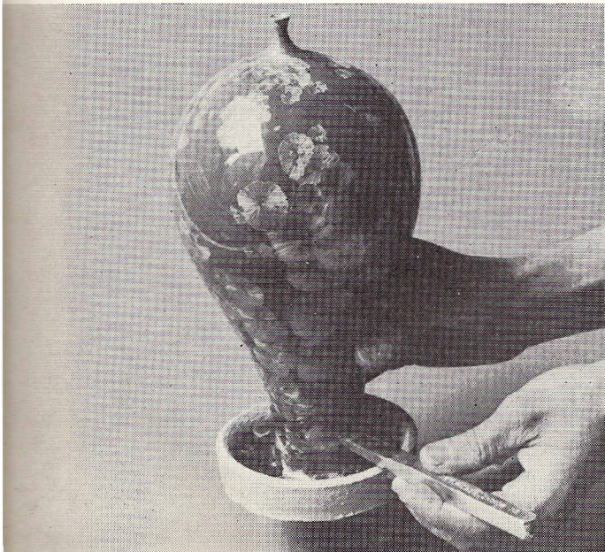
7. By gently tapping with a sharp chisel, the glaze is cleanly fractured at the base to separate the fired form.
