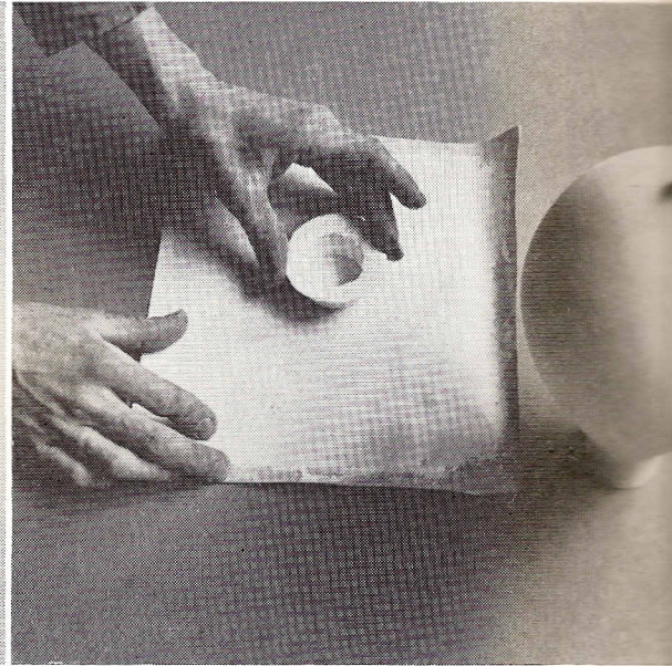
2. To form a tight seal, the ring and base of the pot are ground flat after bisque firing.
